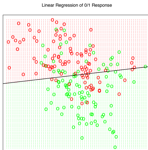
Figure 2.1: A classification example in two dimensions. The classes are coded as a binary variable— GREEN = 0, RED = 1—and then fit by linear regression. The line is the decision boundary defined by x^T \hat{\beta} = 0.5 . The red shaded region denotes that part of input space classified as RED , while the green region is classified as GREEN .
